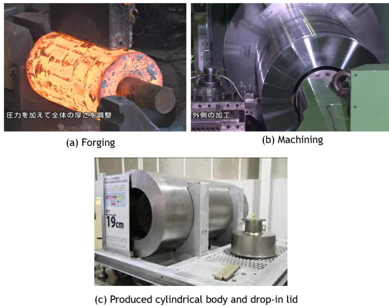
Figure 4.4-7 Production of a carbon steel overpack by forging (Source: (a), (b) [49]; (c) [50])
